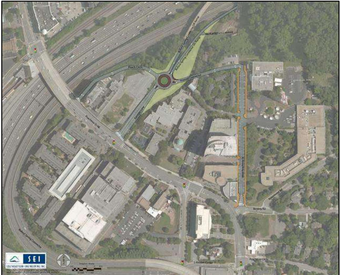
The Build condition for this project considers the installation of a roundabout as shown in Figure 2. SEI has performed peak hour traffic analysis for existing year (2016) conditions, Opening Year (2020) No Build and Build conditions, and Design Year (2040) No Build and Build conditions.
